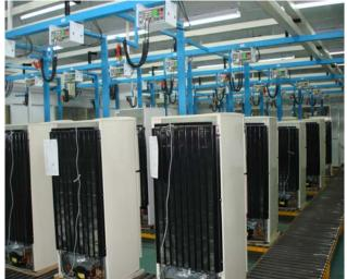
110 nos CPT XD boxes testing 100% of refrigerators for set criteria according to each individual bar coded refrigerator. With real power consumption check, ensure right component usage and performance.
