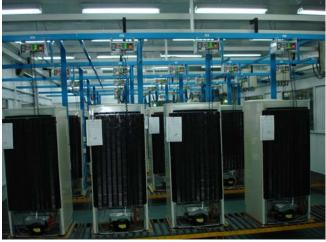
After pass/fail of testing, refrigerators are taken out of the test room with full functional test and next batch of finished refrigerators to be brought in. The CPT XD can be converted to carousel system also.
