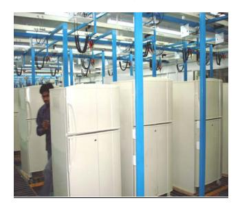
Back view of stand alone system to pass or fail according to set criteria. Agramkow CPT XD boxes are installed in the top of the picture.
