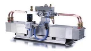
RS-170 Pneumatic supply pump integrated filter solution which is easy and cost-efficient as it is supplied by air only. Pump is "cooled" by air release during every pump stroke to maintain good chillier effect without need for cooling circuit.
