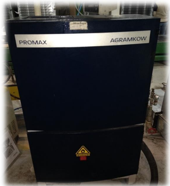
Figure 1: Promax Charging Station for R600a
